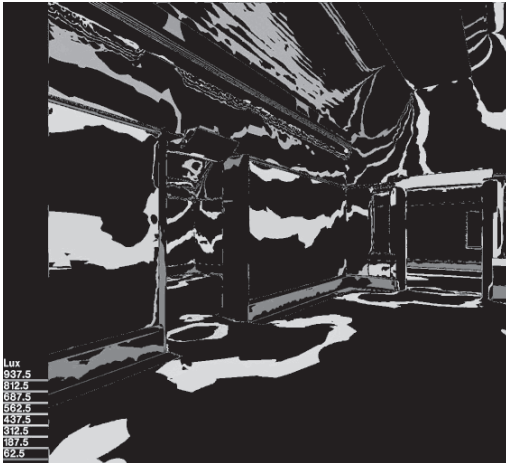
262 Light simulation: false colour intensity analysis in the space of figure 262 (by A.M.J. Post)
