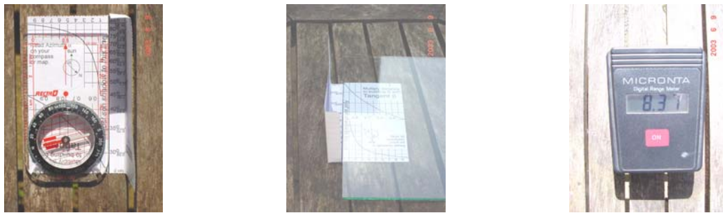
Fig. 49 Measuring Azimuth, sunheight and building height outdoors
