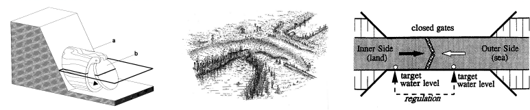
Fig. 469 The oldest one way sluice found in the Netherlands and its modern principle b
