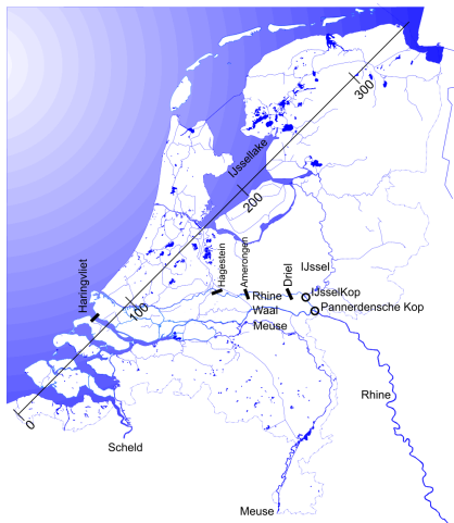
Fig. 441 Weirs directing water northwards and southwards a
